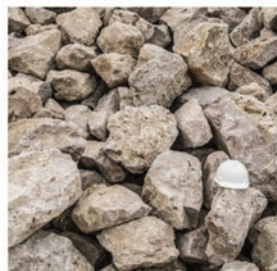
RIP RAP STONE #2 Stone used at the top of the reef ridges; approximate average diameter ranging from 1.25 ft to 3 ft
