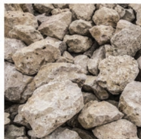
RIP RAP STONE #1 Stone used at the base of the reef ridge; approximate average diameter of 2.5 ft
